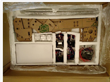
Layer 3 of Printer Parts: Frame parts, power supply, extruder, stepper drive motors, rails, linear bearings.
