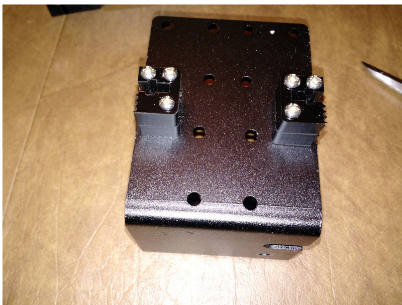
To the extruder's u-shaped carriage holder install two belt holders. These are double plastic parts with teeth to hold the belt.
