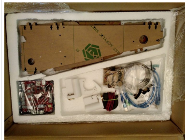
Layer 2 of Printer Parts: Frame parts, z-axis mounts, control board, cooling fans, usb cable.
