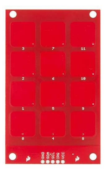
The keypad has 5 lines that need to be connected to your microcontroller, including the power lines, the IRQ line and the  $I^2C$  lines.
